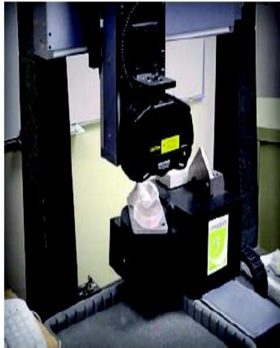
Fig. 2. Laser-scanning of a plaster model with a multi-axis robot to obtain several perspectives (image courtesy of Geodigm, Corp.).
